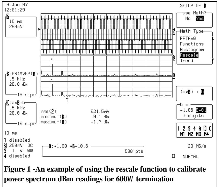
**Figure 1 -An example of using the rescale function to calibrate power spectrum dBm readings for 600W termination**
